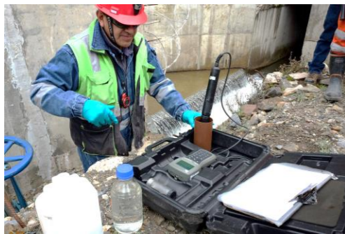
Checking the quality of water discharged into the river from the tailings dam (Huanzala Mine)
