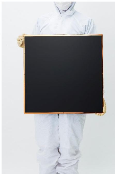
600mm panel type HRDP® product as a work in progress after mold resin encapsulation on a semiconductor package manufacturing process (including Line/Space 2/2 \mu m RDL 4 )
