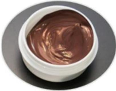
Photo 1: Cu sinter paste
